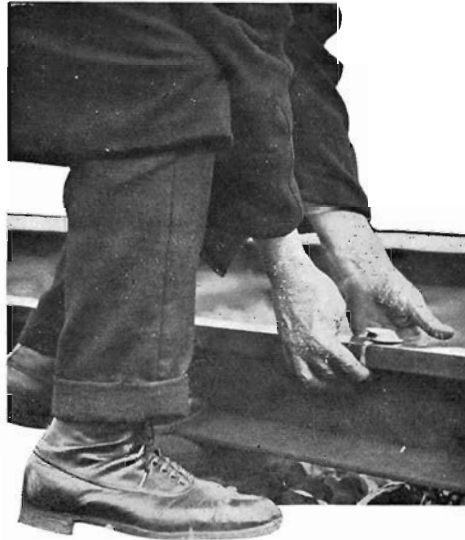
Clamping the warning detonator to the rail
